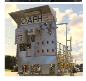
A panel mounted control system comprising of an Ex'd enclosure (with selector switches and start/stop buttons), 515 controller taking density and flow readings received from the Micro Motion Coriolis meter and making real-time adjustments for stroke length and speed of pumps (VSD control) to achieve the correct flow and concentration of diluted product. The VSD panel is located off skid in a safe area.
