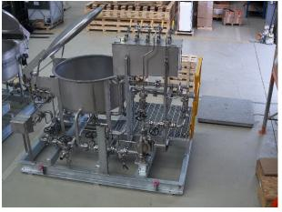
Skid packages delivered with full factory acceptance testing, 316SS materials of construction, intricate tubing (with vent and drain lines), in line with client specification and quality assurance requirements.
