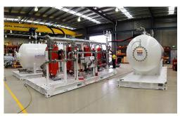
Site design conditions required all equipment rated for cyclonic conditions (with wind speeds over 300km/h). Design verification and proof load testing for lifting/transport were carried out. Other on skid equipment included, 316SS piping, instrumentation, pressure control valves, pressure relief valves and electrical control stations.
