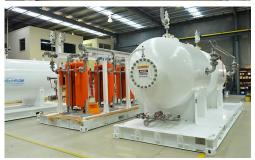
Instrument Air System comprised of 4 off 90kW compressors, 2 off wet receiver vessels and 1 off dry receiver vessel (to AS1210) and a dryer package. Modular design in total 5 off 20ft modified shipping containers and bases with interconnecting pipework.
