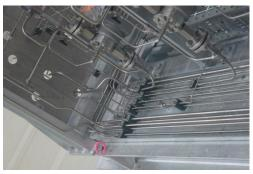
Skid package delivered with full factory acceptance testing, 316SS materials of construction, intricate tubing (with vent and drain lines), in line with client specification and quality assurance requirements.
