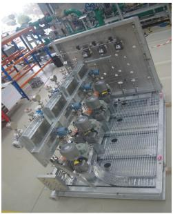
This style of pump is electrical motor driven with system functionally allowing for flow rate adjustment via electronic stroke length changes (4 to 20mA signal) and/or via an external VFD which can vary the motor speed providing accurate flowrate turndown.
