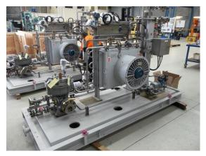
Scope included dual unpressurised tandem process seal arrangement - monitored by the plan 52 seal system via the pressure and temperature transmitters and gauges. Secondary seal leakage will also be to the plan 52 system. A pressurised lube oil system consisting of an external pre-lube oil pump and a forced draft, pin fin air cooler is fitted to the pumps. (2 off skids supplied in total)
