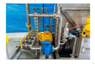
Package included hydraulic power pack driving hose reel (controls on both sides depending on operator line of sight), emergency breakaway couplings, emergency release couplings (hydraulically activated), control cabinet contained all mounted within a fully self bunded base frame tank.
